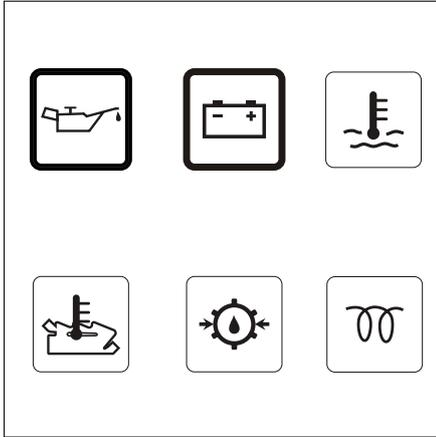
**Monitoring lights oil pressure and battery charging current**
