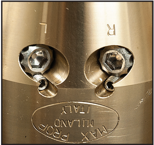
Fig.5 - Close up of the Left and Right pitch adjustment bolts.
